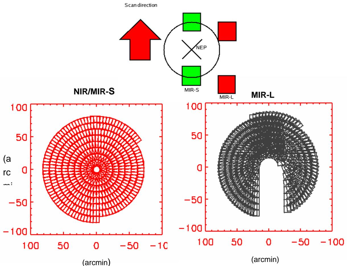
Figure 2. "NEP-Wide" mapping strategy when the survey is done only in Phase-1. IRC has two FOVs: NIR/MIR-S and MIR-L, separated by 20 arcmin. Thus, if NIR/MIR-S uniformly covers the circular area (bottom, left), MIR-L coverage is no longer uniform (bottom, right). (prepared by S. Oyabu)
