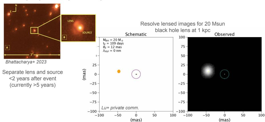
Diffraction limit on 8-10 m telescopes is 15-20 mas in the visible. Use Subaru ULTIMATE-START to explore atmospheric tomography algorithms needed for future visible-light AO systems (eg KOLA at Keck).
