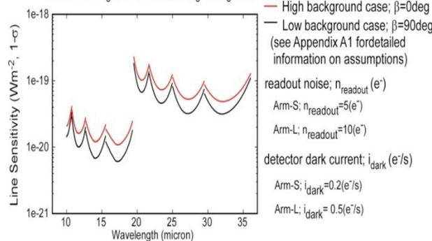
MIRMES Line Sensitivity for Extended Source, 1-sigma for 600 sec integration time at low & high background
