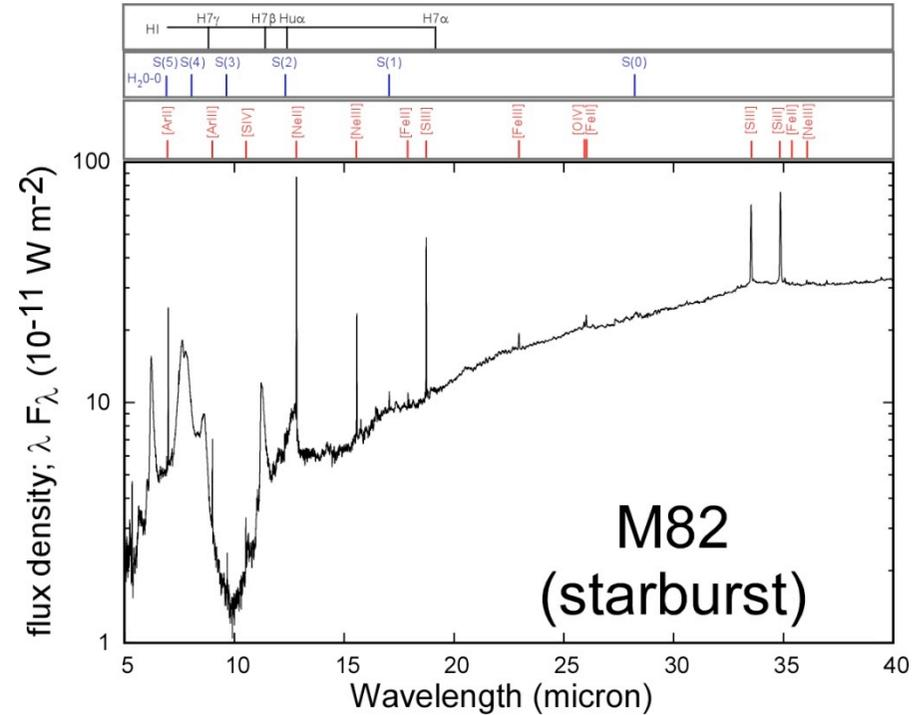
ionized gas ; [NeII] 12.81 $\mu$ m, [Ne III] 15.56 $\mu$ m, 36.01 $\mu$ m, [NeV] 14.32  $\mu$ m, [S III] 33.48 $\mu$ m, 18.71 $\mu$ m,
