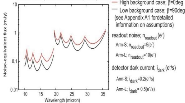
MIRMES Line Sensitivity for Point Source, 1-sigma for 600 sec integration time at low & high background
