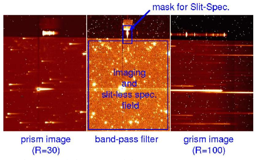
An example of slit-less and slit spectroscopic images obtained by AKARI/IRC.
